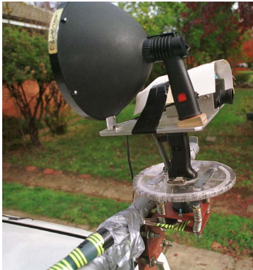
Figure 7.1: Line-transect equipment. To increase the rate of recording observations at night, the spotlight, laser rangefinder and compass rose were mounted on a commercially available ball and socket device (seen here with grip handle and locking lever) in such a way they could be finely adjusted to co-align. A red laser beam (not visible) marked the ‘zero’ point where the bearing on the compass rose was read, with the aid of a small light to illuminate the engraved digits. A white plastic cover protected the rangefinder from light rain or snow. Twelve coil springs (visible below the compass rose) insulated the equipment from both engine vibration and shocks due to the vehicle bumping over rocks.
