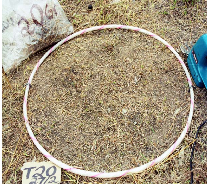
Figure 5.4: A clipped plot in grazed pasture. Additional disc meter readings were taken after clipping (as well as before) to consider the effect of terrain on the disk meter.
